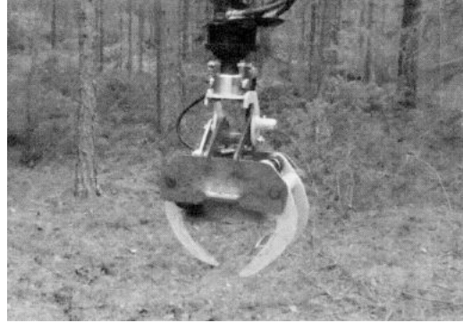
2. When jaws are opening the grapple starts to move into UP position.
