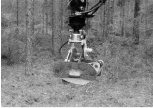
1. Jaws fully closed the grapple is in DOWN position.
