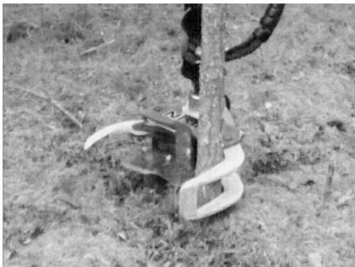
5. The jaws are kept open until the tree is positioned as seen in the picture.
