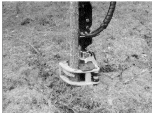
6. The cut is made by closing the jaws.
